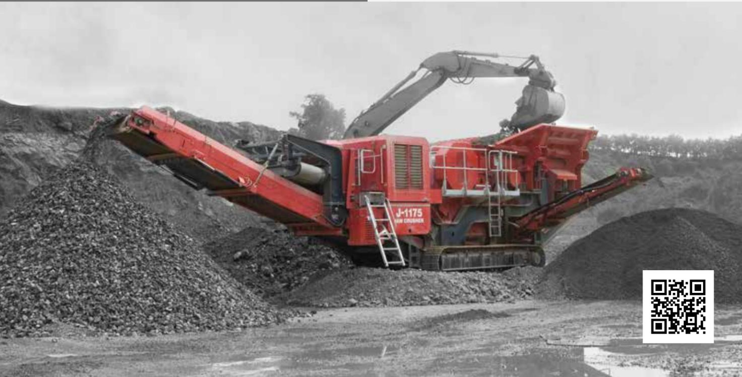
The Finlay® J-1175 mobile Jaw Crusher is a high performance and aggressive primary crushing plant for medium sized operators in quarrying, demolition, recycling, and mining applications.
