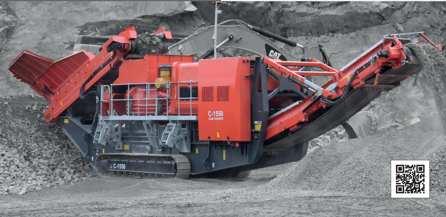
The Finlay® C-1550 mobile cone crusher is a high capacity and aggressive machine for the surface ore mining and aggregate industries.
