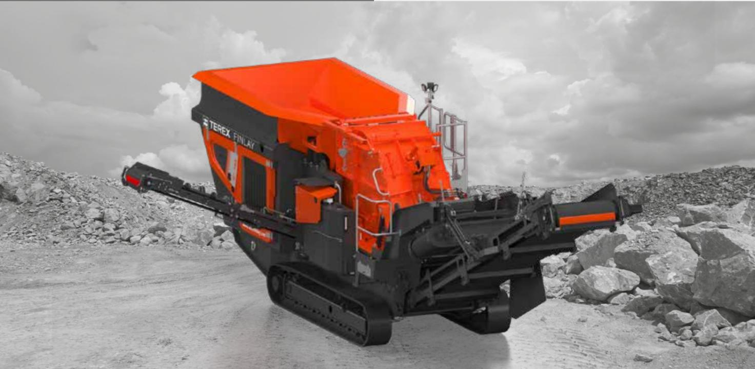
The Finlay® IC-100 mobile impact crusher has been specifically designed for quarrying, construction and demolition debris, reinforced concrete and asphalt recycling applications.
