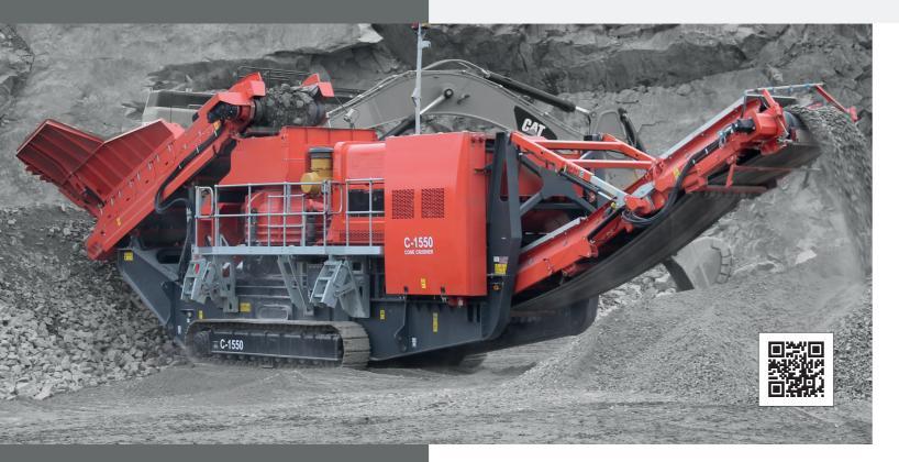
The Finlay<sup>®</sup> C-1550 mobile cone crusher is a high capacity and aggressive machine for the surface ore mining and aggregate industries.
