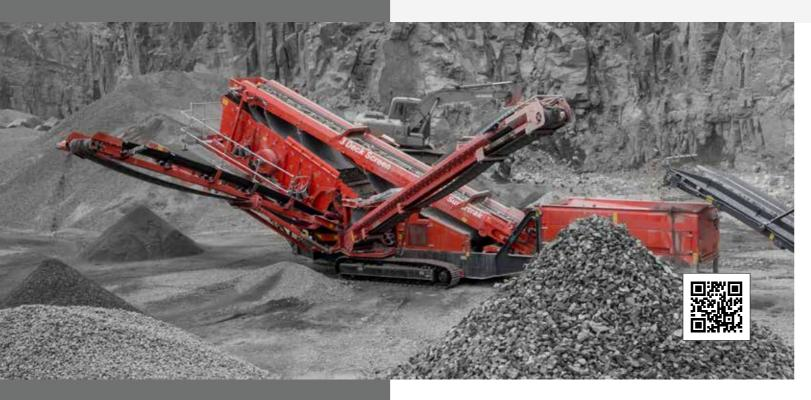
The Finlay<sup>®</sup> 684 3-Deck inclined screen is a compact easily transportable machine that offers operators rapid set up and tear down times.
