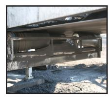
The Tri-Return Training Idler<sup>®</sup> eliminates belt and structure damage caused by misalignment.
